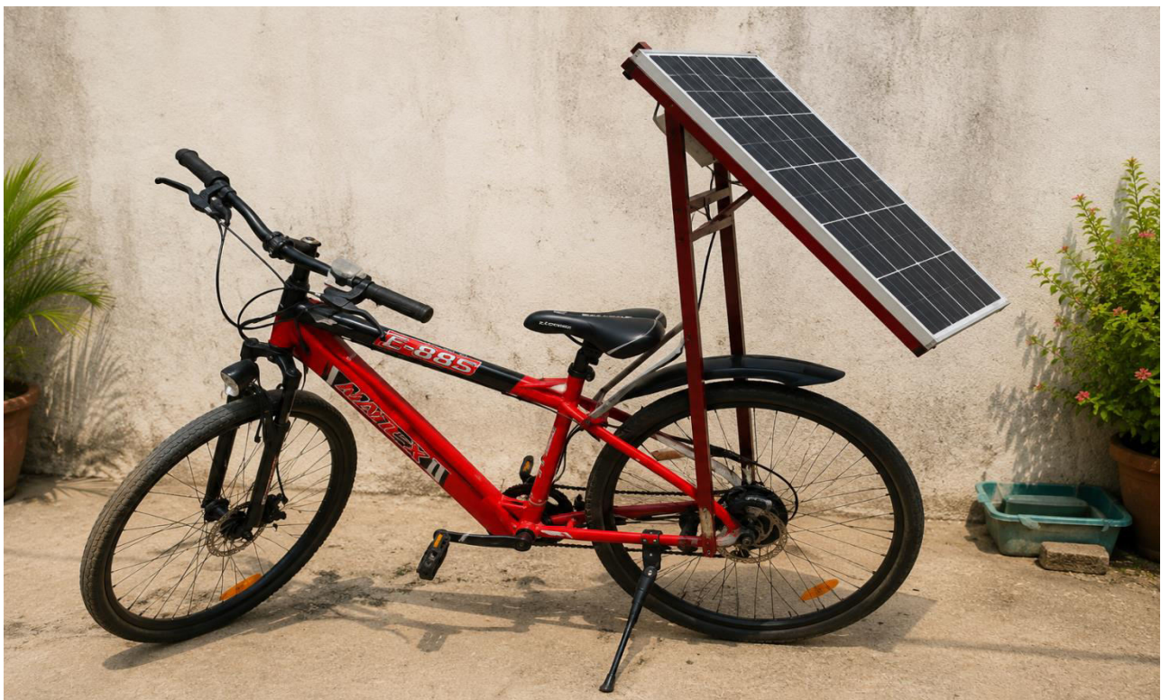
Figure 4.1 (a) Final Model of Development of Eco-Friendly Hybrid E-Bicycle Using Renewable Energy Sources
